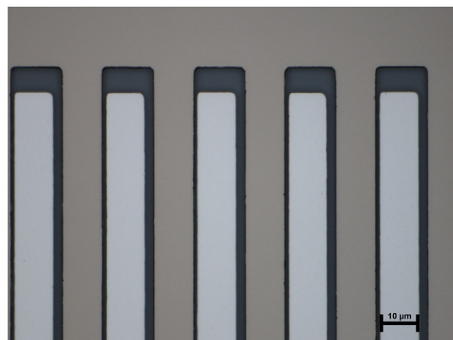
Fig. 2. 100 \times magnified image of the interdigitated 2 metal electrode substrate.
