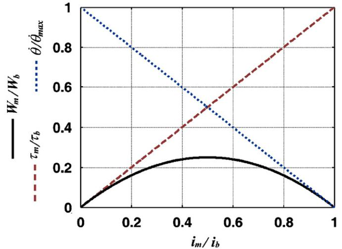
Fig. 2. DC motor characteristics.
