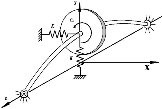
Fig. 1. A Symmetric rotor-shaft system with spinning speed  $\Omega$ . The stiffnesses of the shaft and the internal and external damping are referred to the rotor disk.
