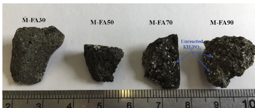
Fig. 1. Fractured surface of the FA blended MKPC mortars cured in air (23 °C and 65% R.H.) for 28 days.
