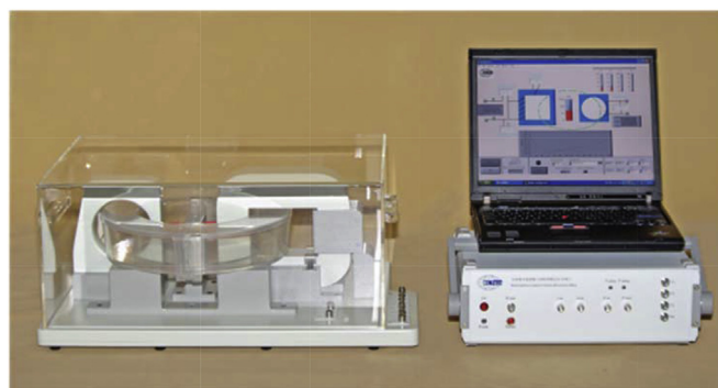
Fig. 2. The system for electrodeless resistivity measurement.
