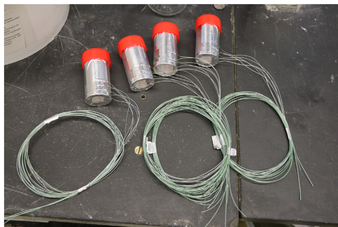
Fig. 2. Molds with thermo-couple wires.
