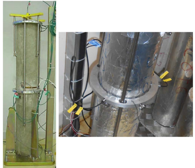
Fig. 2. Left: 1D drying shrinkage test in the creep tests room at CEIDRE-TEGG. Right: zoom on the radial measurement ring for a 1D non-drying shrinkage test.
