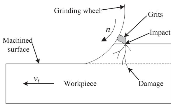
Fig. 1.1. Abrasive machining processes.
