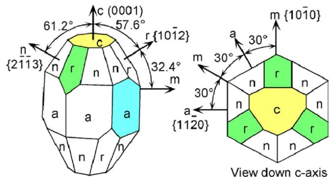
Fig. 2.1. Crystallographic diagram of sapphire [1].
