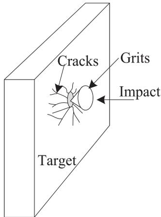
Fig. 1.2. Crack propagation under impact loading.
