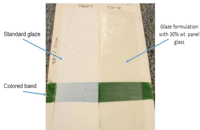
Fig. 1. The unfired ceramic substrate with the applied green band; test and standard glaze layers on engobe.
