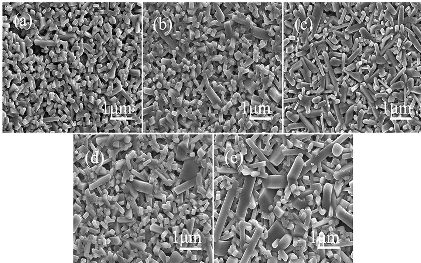
Fig. 2. SEM of different samples (A) SEM of  $\text{Na}_{1+x}\text{BiTi}_6\text{O}_{14+0.5x}$  ( $x = 0.01$ ) ceramics sintered at various sintering temperature ( $T = 1000, 1020, 1040, 1060, 1080^\circ\text{C}$ ), (B) SEM of  $\text{Na}_{1+x}\text{BiTi}_6\text{O}_{14+0.5x}$  ( $x = -0.02, -0.01, 0.01, 0.02$ ) ceramics sintered at  $1040^\circ\text{C}$ .
