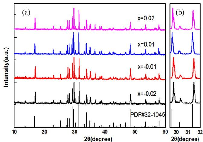
Fig. 1. X-ray diffraction patterns of  $\text{Na}_{1+x}\text{BiTi}_6\text{O}_{14+0.5x}$  ( $x = -0.02, -0.01, 0.01, 0.02$ ) samples sintered at  $1040^\circ\text{C}$  (a)  $10\text{--}70^\circ$ , (b)  $29.5\text{--}32^\circ$ .
