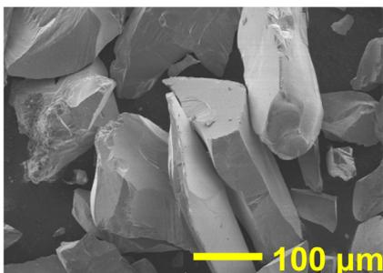
Fig. 1. The SEM image of SiC particles.
