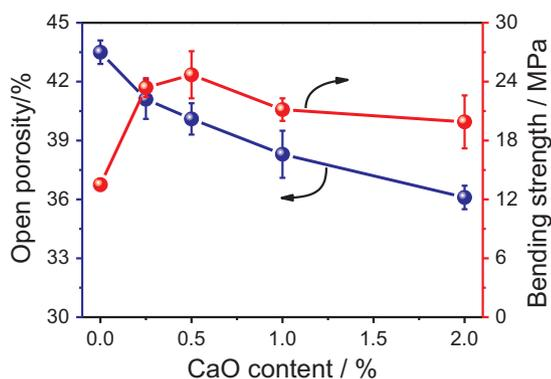
Fig. 3. The open porosity and bending strength of RBSC porous ceramics changed with CaO content.
