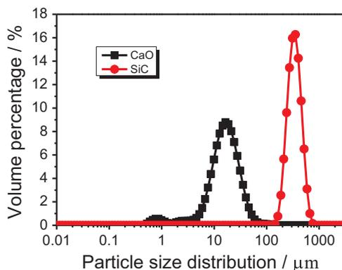
Fig. 2. The particle size distribution of both CaO and SiC.
