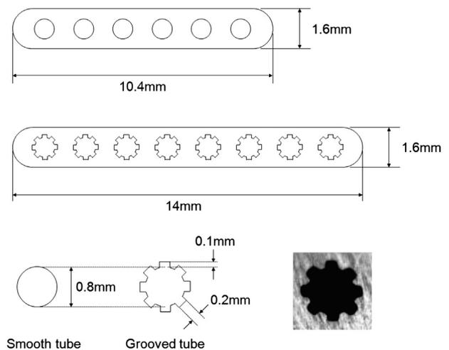
Fig. 1 – Cross section of the tested mini tubes (unit: mm).
