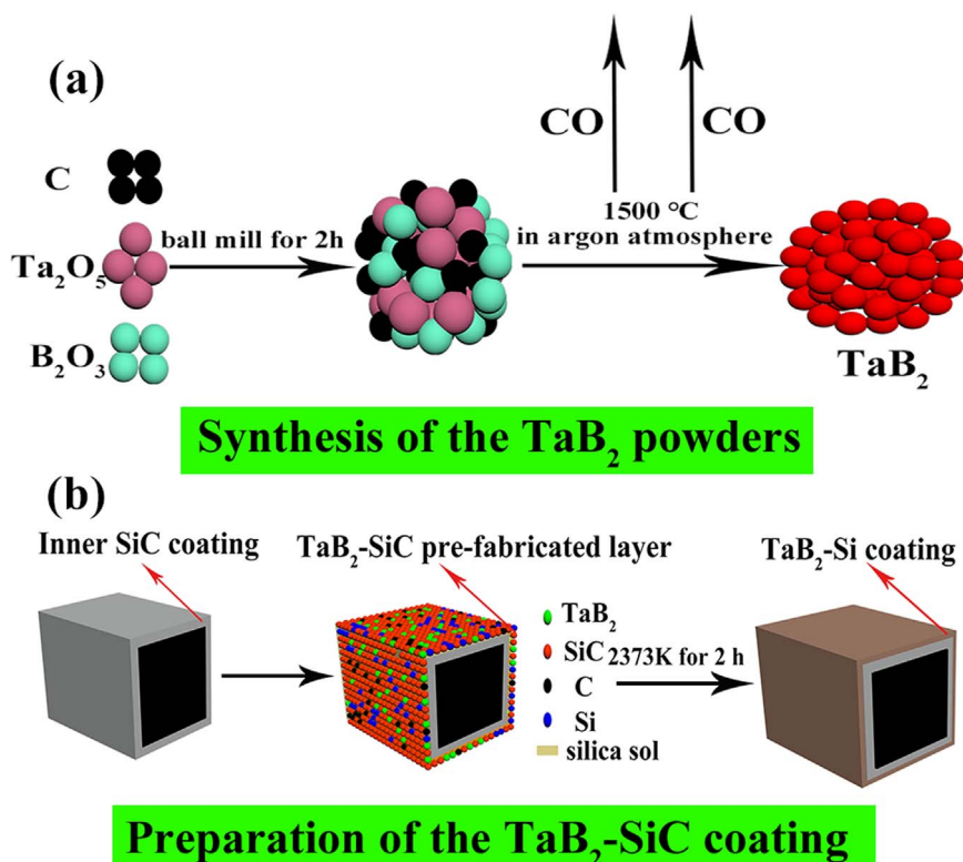
Fig. 1. Illustration of the preparation of the TaB 2 powders (a) and the outer TaB 2 -SiC coating (b).
