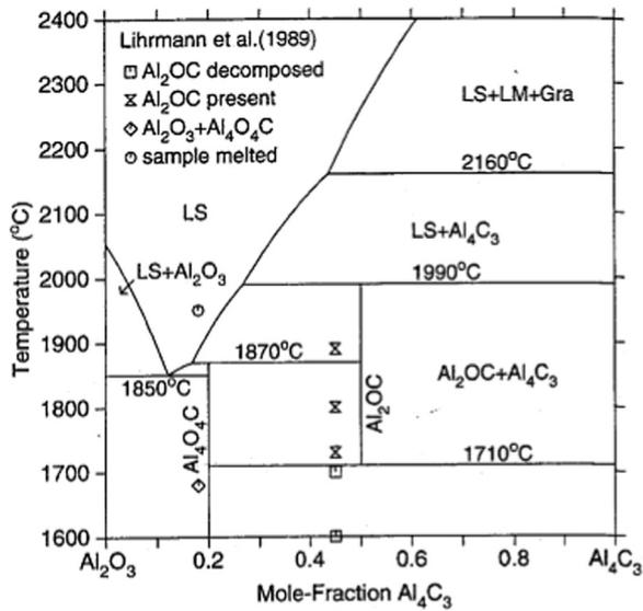
Fig. 1. Calculated phase diagram of the pseudo-binary  $\text{Al}_2\text{O}_3\text{-Al}_4\text{C}_3$  system of Qiu and Metselaar [22] in comparison with experimental observation of Lihmann et al. [23].
