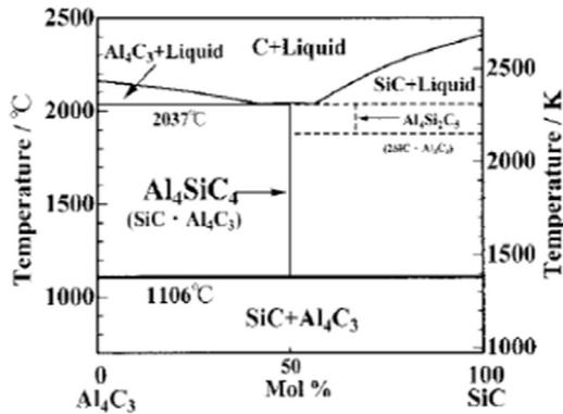
Fig. 2. Calculated phase diagram of the pseudo-binary  $\text{Al}_4\text{C}_3\text{-SiC}$  system [26,27].
