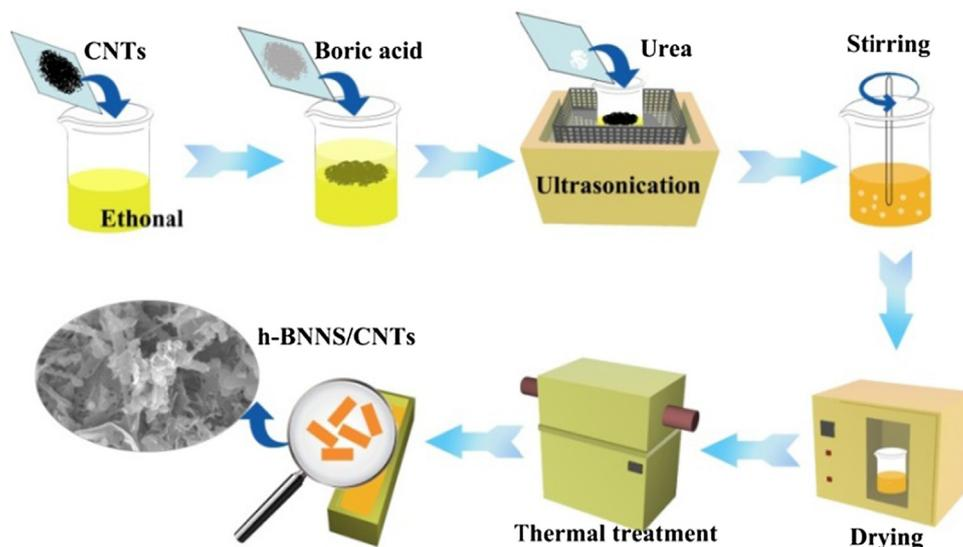
Fig. 1. Schematic illustration for the fabrication of *h*-BNNS/CNT composites. (For interpretation of the references to colour in this figure legend, the reader is referred to the web version of this article.)
