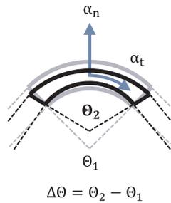
Fig. 1. Spring-in of a curved composite laminate. (For interpretation of the references to colour in this figure legend, the reader is referred to the web version of this article.)
