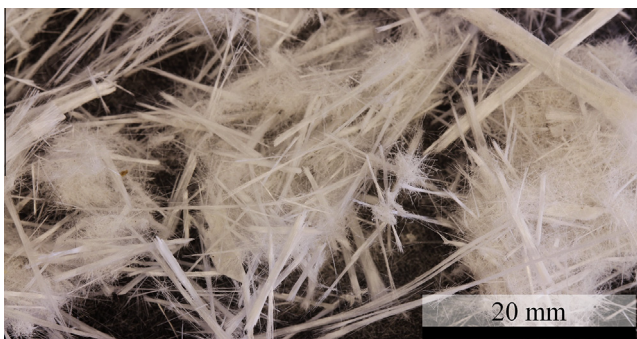
Fig. 2. Shredded composite. (For interpretation of the references to colour in this figure legend, the reader is referred to the web version of this article.)
