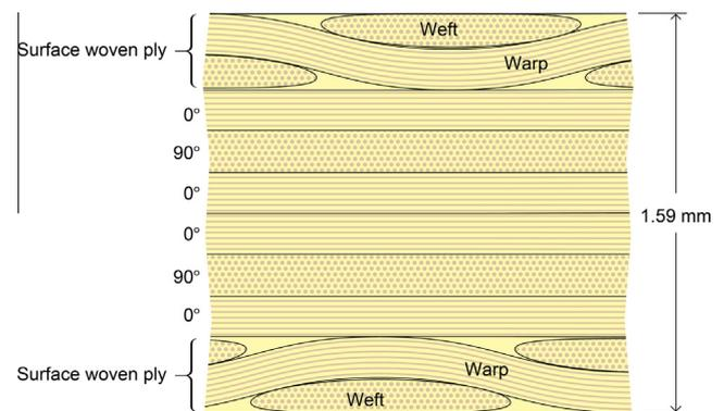
**Fig. 2.** Schematic illustration of the internal structure of the as-received CFRP laminate used to make the lattice. The laminate comprised 2 surface plies made from plain weave fabrics that sandwich 6 unidirectional plies of the same thickness arranged as a [0/90/0]s layup. (For interpretation of the references to color in this figure legend, the reader is referred to the web version of this article.)
