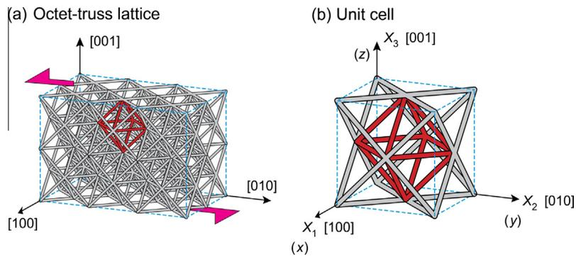
**Fig. 1.** (a) An octet-truss lattice constructed by the 3D translation of the unit cell shown in (b). The unit cell of the octet-truss lattice is composed of a (red) center octahedral unit and 8 (gray) edge tetrahedral cells. (For interpretation of the references to color in this figure legend, the reader is referred to the web version of this article.)
