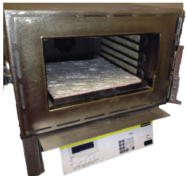
Fig. 1. Photo of 16 layers of chopped strand mat heat-conditioned in the furnace. (For interpretation of the references to colour in this figure legend, the reader is referred to the web version of this article.)
