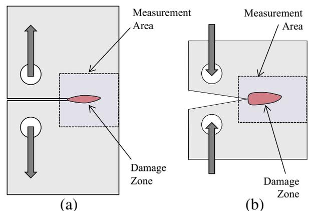
**Fig. 1.** (a) Schematic of the over-height compact tension (OCT) test; and (b) schematic of the compact compression (CC) test. (For interpretation of the references to colour in this figure legend, the reader is referred to the web version of this article.)
