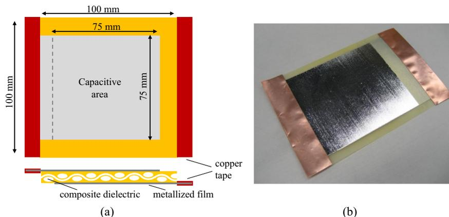
Fig. 2. (a) Schematic and (b) photograph of unencapsulated capacitors, sets 1–7. (For interpretation of the references to colour in this figure legend, the reader is referred to the web version of this article.)
