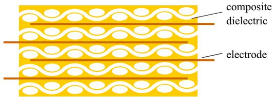
Fig. 1. Schematic of a structural capacitor. (For interpretation of the references to colour in this figure legend, the reader is referred to the web version of this article.)
