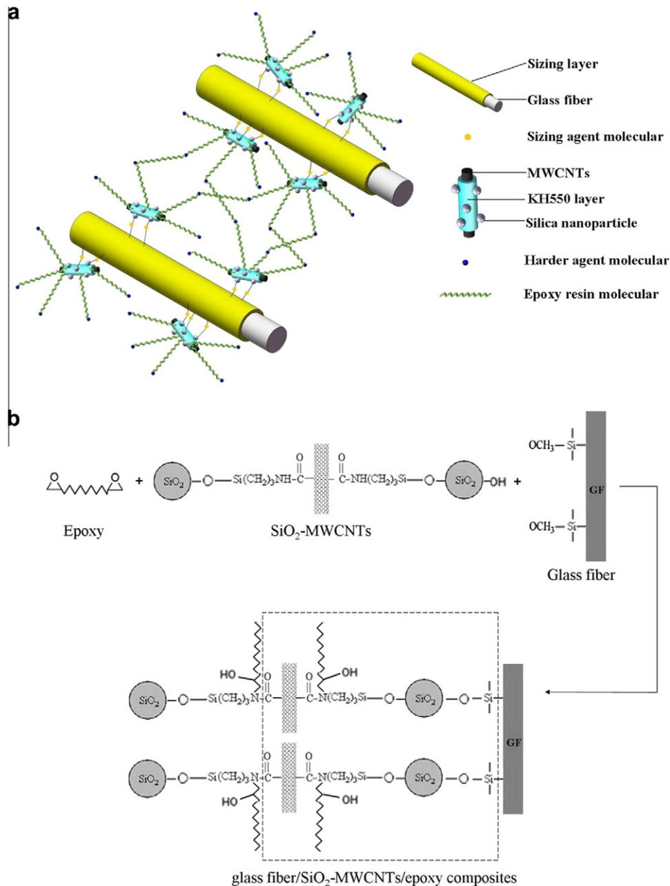
**Fig. 1.** Schematic of (a) microstructure and (b) interfacial chemical reaction of GF/EP composites with silica nanoparticle-multiwalled carbon nanotube (SiO<sub>2</sub>-MWCNT) complex. (For interpretation of the references to colour in this figure legend, the reader is referred to the web version of this article.)
