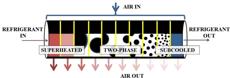
Fig. 1 – FV model with 10 control volumes for a cross-flow refrigerant-to-air condenser.
