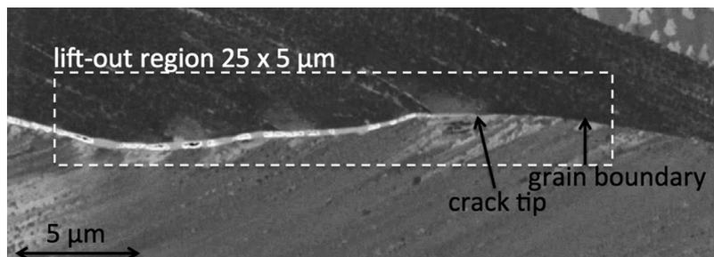
**Fig. 1.** FIB image (FEI FIB200) of intergranular stress corrosion crack in stainless steel specimen: a region of 25 μm × 5 μm has been selected for lift-out; both crack tip and grain boundary are indicated.
