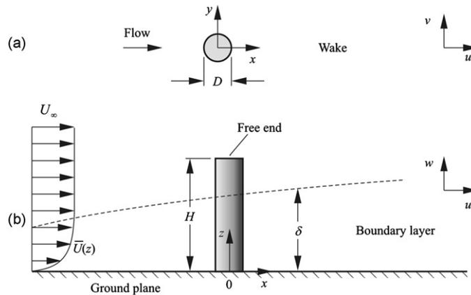
**Fig. 1.** A schematic representation of flow past a finite circular cylinder mounted normal to a ground plane and partially immersed in a flat-plate boundary layer: (a) top view and (b) side view.
