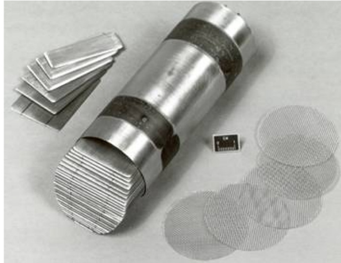
Fig. 1 – First room-temperature magnetic heat pump designed in 1976 by G. V. Brown (Brown, 1976; Gschneidner and Pecharsky, 2008).
