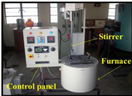
Fig. 1. Casting facility used to prepare Al6101/Graphite AMCs.
