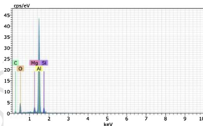
Fig. 1. EDX analysis showing percentage of AA5083 reinforced with 1.25wt% of MWCNT.
