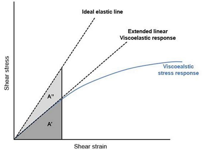
Fig. 3. Area showing viscos and elastic effect of material in shear stress vs shear rate graph.
