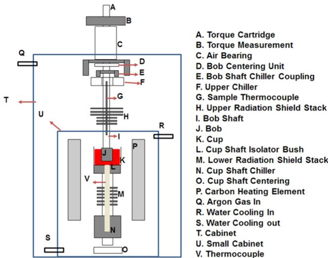
Fig. 2. Schematic depiction of rheometer equipped with high temperature furnace. (Ravenfield Modle FG MkIV; Ravenfield Designs Ltd., Heywood, UK).
