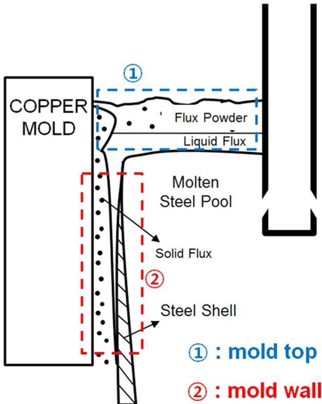
Fig. 1. A schematic diagram of mold area for continuous caster.
