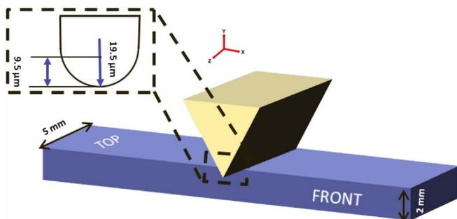
Fig. 2. Schematic of wedge indentation setup for SB observation with wedge dimensions.
