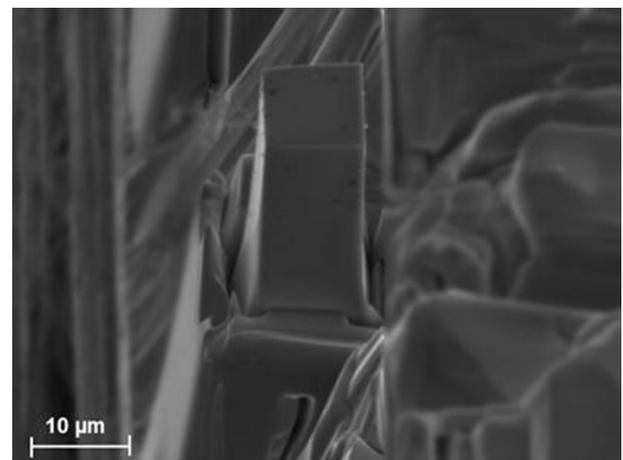
Fig. 3. Micropillars of as-fabricated  $Zr_{48}Cu_{36}Al_8Ag_8$  with square cross-section of 10  $\mu\text{m} \times 10 \mu\text{m}$ .
