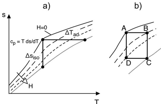
Fig. 1 – a) Entropy state equation  $s(H, T)$ . b) Magnetic Carnot cycle in the  $(s, T)$  diagram.
