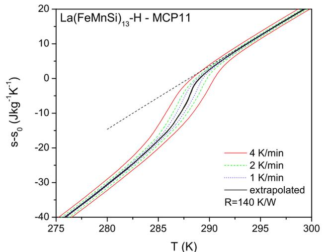
Fig. 2 –  $\text{LaFe}_{11.384}\text{Mn}_{0.356}\text{Si}_{1.26}\text{H}_{1.52}$  powder of mass 109.95 mg measured by heat compensation calorimetry under different rates. Sample entropy  $s$  by Eq. (1). The extrapolated curve is obtained by using  $T_s$  of Eq. (2) with  $R = 140 \text{ kW}^{-1}$ .
