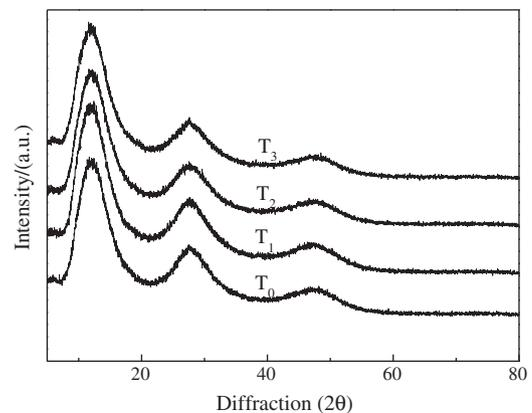
Fig. 2. XRD pattern of the powdered glass samples.
