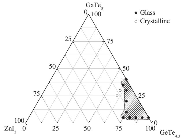
Fig. 1. Glass-forming region of Ge–Ga–Te– $\text{ZnI}_2$  system.
