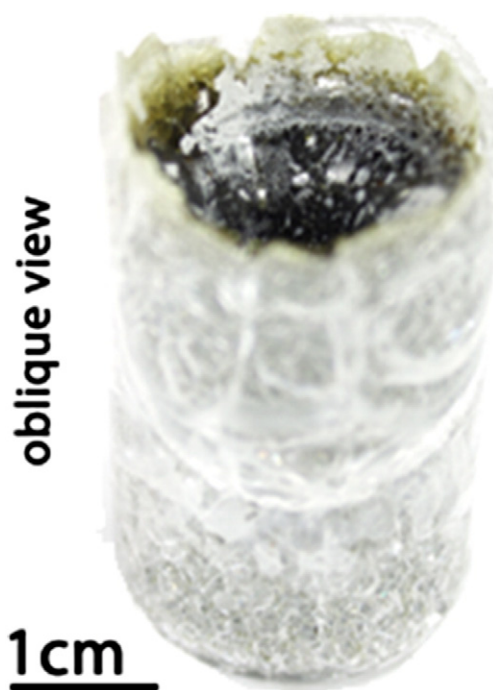
Fig. 1. Heat treated sample remaining after the upper part of the fused silica ampoule wall is broken off along the boundary of the glass (at the meniscus of glass melt).
