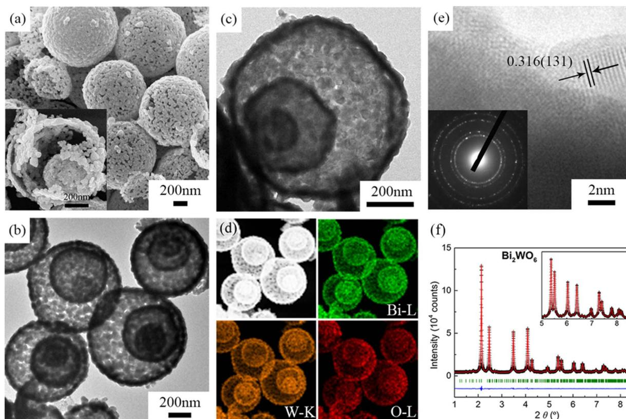
Fig. 1. (a) and (b) SEM and TEM image of BWO-MSH. (c) and (e) HRTEM images of the BWO-MSH. The inset of (e) is selected area electron diffraction. (d) HAADF-STEM element mapping. (f) SXR D pattern of the microspheres. The inset is an enlargement of high angle region.
