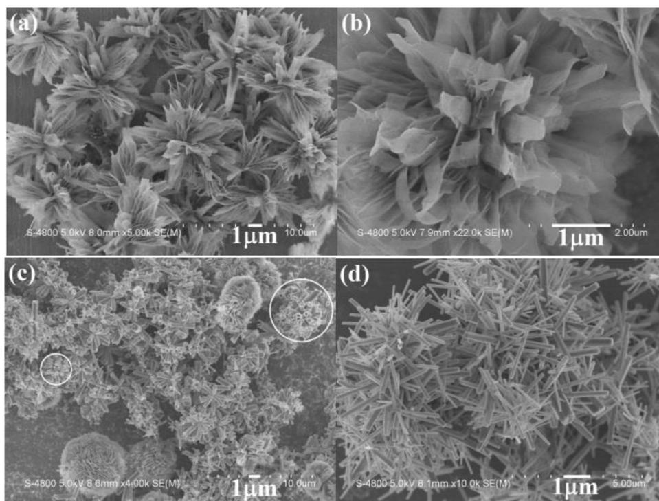
**Fig. 2.** SEM images of the products prepared from the present reflux system at 120 °C for different reaction durations: (a, b) 30, (c) 90 and (d) 120 min.
