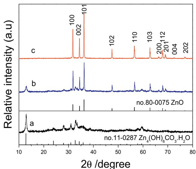
**Fig. 1.** XRD patterns of the products prepared at 120 °C for different reaction durations: (a) 30, (b) 90 and (c) 120 min.
