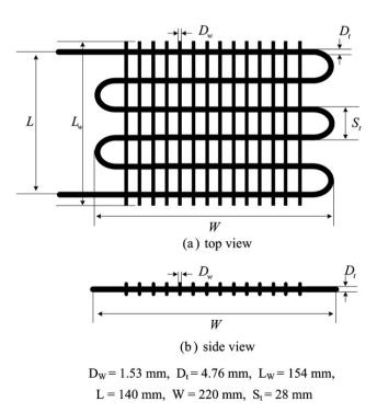
Fig. 1 - The single layer of wire-on-tube sample.
