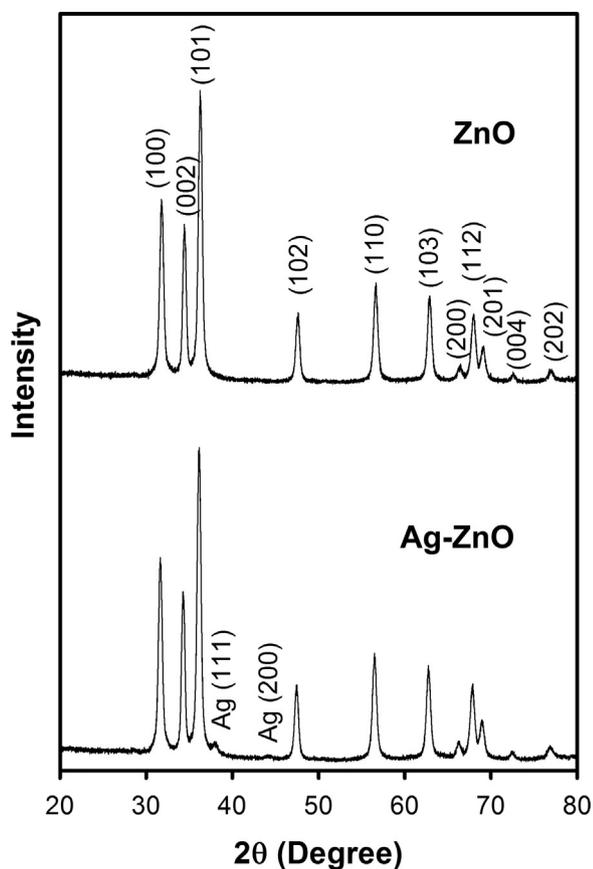
Fig. 1. XRD patterns of ZnO and Ag/ZnO nanoparticles.
