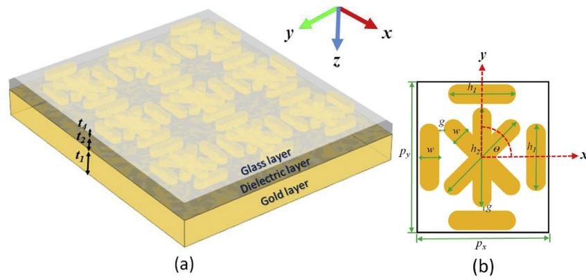
Fig. 1. (a) Schematic of tri-layer metasurface absorber. (b) Unit cell of the resonator.
