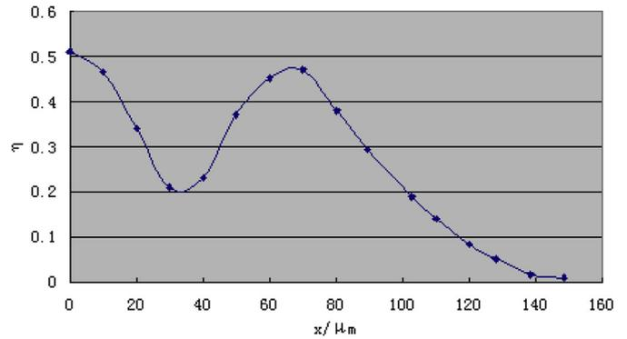
Fig. 3. Coupling efficiency of conical fiber array.
