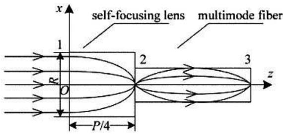
Fig. 1. Coupling model of space light into fiber. 2, 2 The efficiency numerical calculation of conical fiber array.
