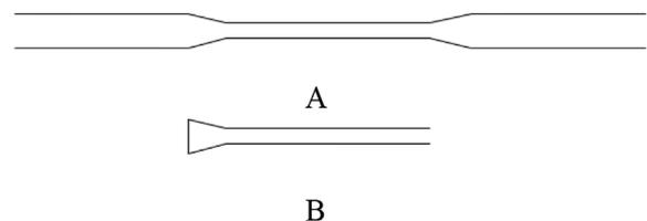
Fig. 4. The process of making a conical fiber.
