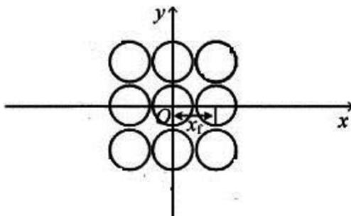
Fig. 2. The distance of  $x_f$  in the conical fiber array.
