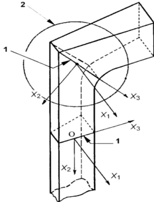
Fig. 1. Supporting line segments definition [4].
