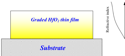
Fig. 1. The physical model of the film-substrate system.
