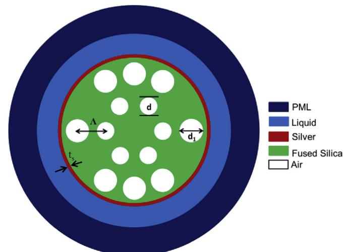
Fig. 1. Cross-section view of the proposed circular lattice PCF sensor with  $\Lambda = 2 \mu\text{m}$ ,  $d = 0.57\Lambda$ ,  $d_1 = 0.78\Lambda$  and  $t_s = 30 \text{ nm}$ .
