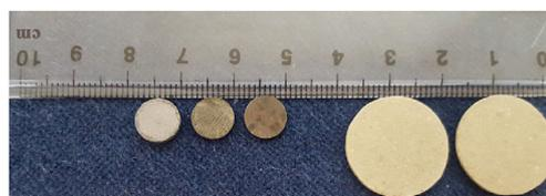
Fig. 1.  $SrS:Ce, Sm$  pellet samples prepared by sintering of the synthesized powders using the SPS method.
