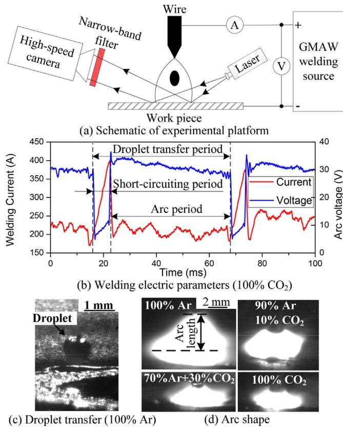
Fig. 1. Observation of droplet transfer and arc shape.
