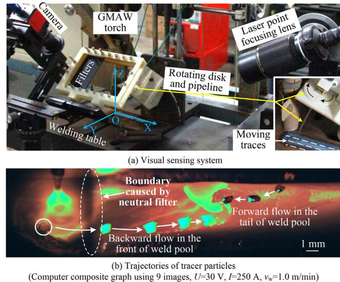
Fig. 2. System used to observe fluid flow on weld pool surface in GMAW process.
