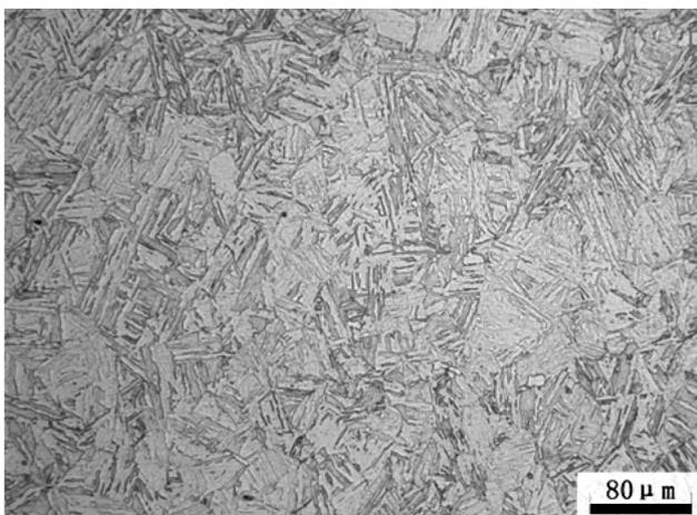
**Fig. 1.** Metallographic structure of FV520(B) steel with optical microscope.
