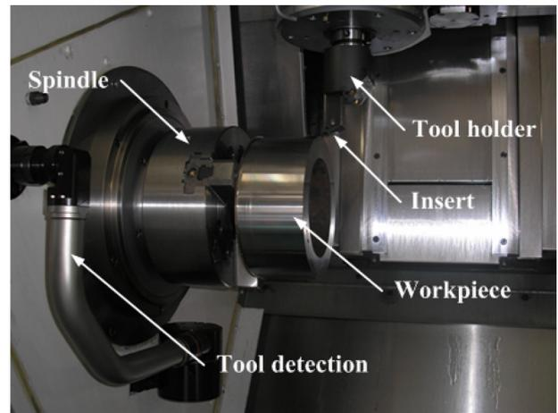
**Fig. 2.** General arrangement of high-speed machining setup.
