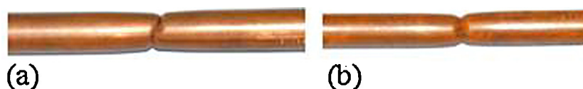
Fig. 3. Copper tubes after tension test: (a) \phi 8 tube and (b) \phi 6 tube.
