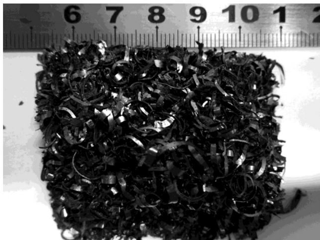
Fig. 1. External appearance of the iron scraps.
