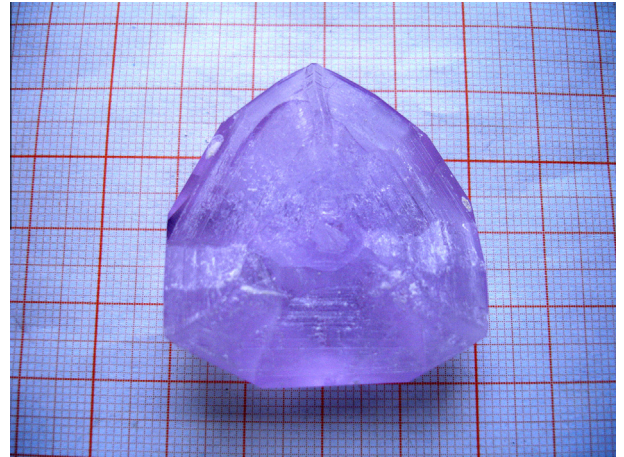
Fig. 1. The grown \text{Nd}^{3+}:\text{Sr}_6\text{YSc}(\text{BO}_3)_6 crystal.
