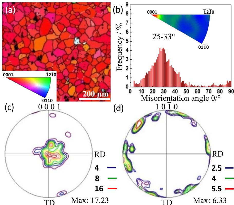
Fig. 1. Microstructure and texture of the solution sample: (a) EBSD map; (b) misorientation angle distribution map; (c)  $\{0001\}$  and (d)  $\{10\bar{1}0\}$  pole figure.
