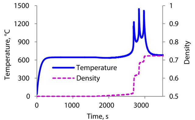
Fig. 1. Simulated temperature and relative density vs. time during microwave heating of a nickel powder compact. Frequency 2.45 GHz, initial radius of compact 1 cm, radius of nickel particles 1 μm, thickness of the oxide layer on particles 2.5 nm. The intensity of the incident microwave radiation 510 W/cm<sup>2</sup>.
