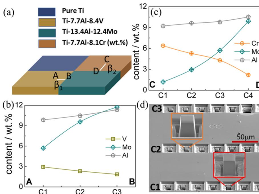
**Fig. 1.** (a) Schematic drawing of diffusion multiple where the selected  $\beta_1$  and  $\beta_2$  interdiffusion regions are indicated; (b), (c) composition of the selected alloys within interdiffusion regions  $\beta_1$  and  $\beta_2$ ; (d) SEM micrograph illustrating the micropillars milled within region  $\beta_1$ .
